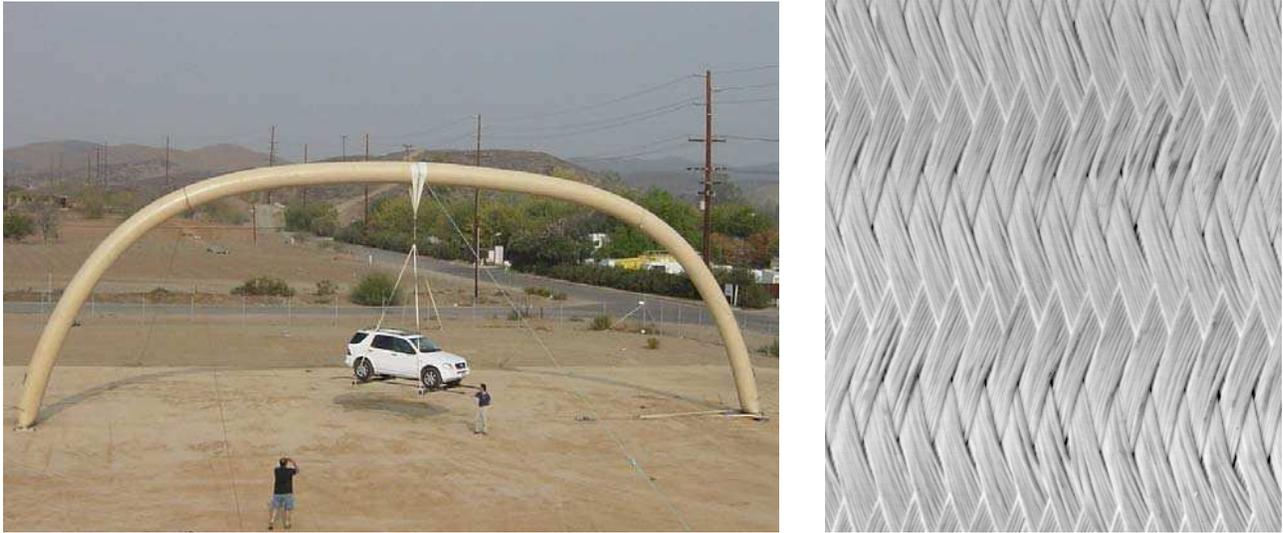
**Figure 1. High Strength AirBeam and Reinforcing Fiber**
