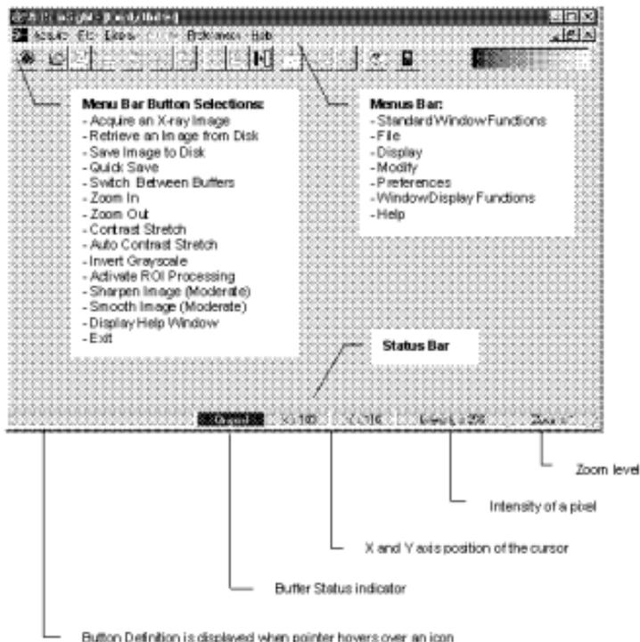
Figure 2.7 ARS User Interface Main Menu screen showing menu bar on the top, icons bar below, and status bar at the bottom.
