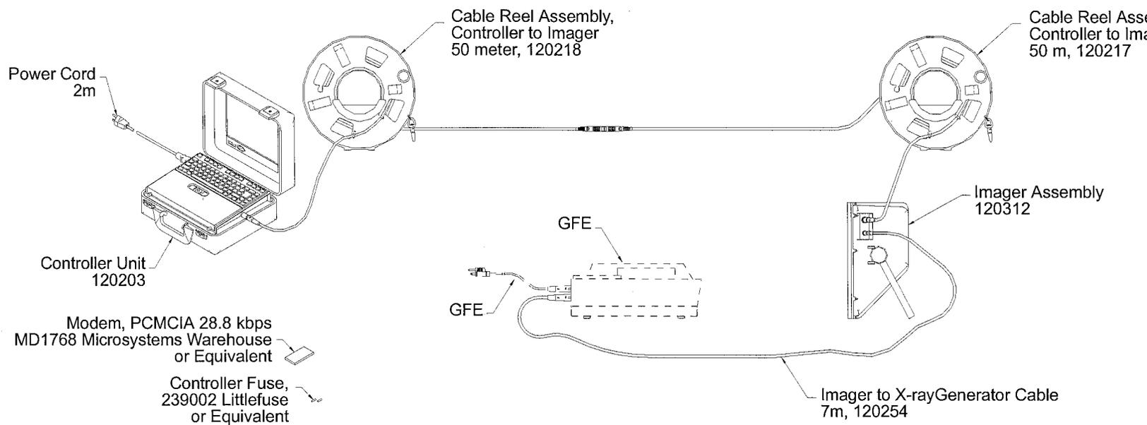
**Figure D1 ARS Standard Components Diagram.**
