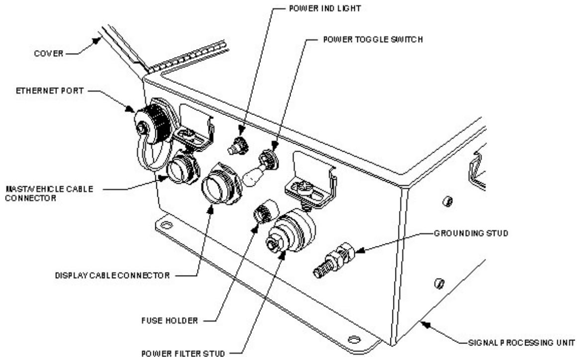
*Figure 8: Boomerang Electronics Box showing power switch, power indicator light, fuse, and cable connectors.*
