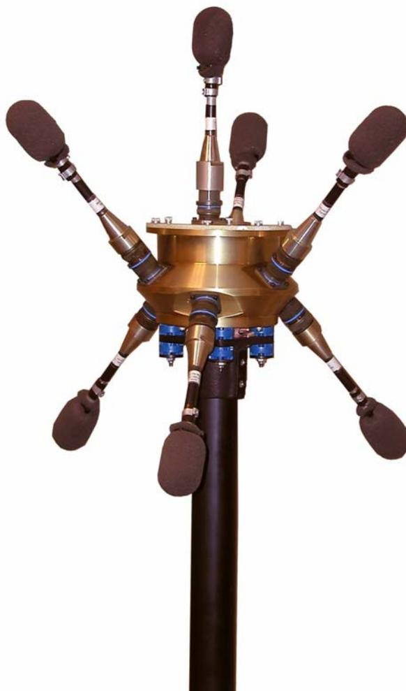
*Figure 2 – Microphone Array, Hub, and Mast Assembly*
